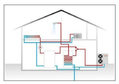
Figure 5: Example Diagram of Air Source Heat Pump Layout
