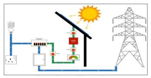
Figure 6: Example Diagram of Solar PV Layout
