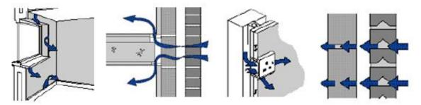
Figure 3: Typical Air Leakage Paths
